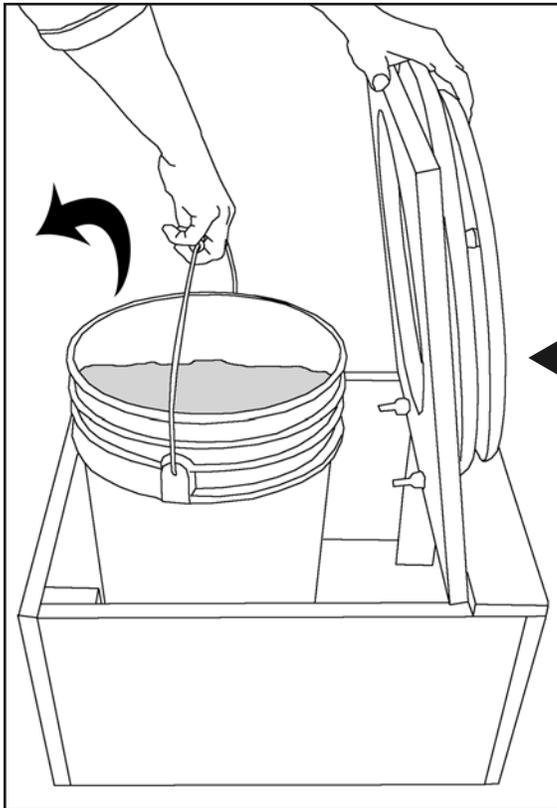
If the toilet receptacle is full, lift plywood lid, remove receptacle, put on plastic lid, and set the receptacle aside for collection and composting.
