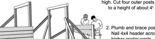
2. Plumb and brace posts. Nail 4x4 header across higher center posts.
